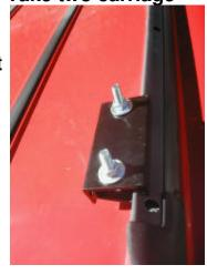
picture to the right. Add a flat washer to each carriage bolt, and then a nut. Tighten down the nuts finger-tight to hold everything in place. Do the same to the other side of the Jeep, and position the bar forward/rearward as you prefer. The further rearward, the less glare on your hood, and the less wind noise you'll get, which is typically noticeable only if you have a moonroof, and sometimes not even then. Lastly, tighten down the
